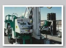
Single station control and wing around auger rack
